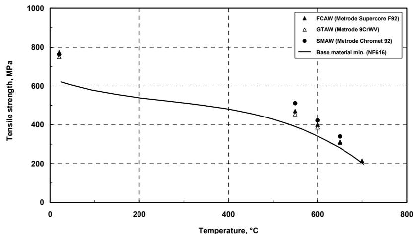
**Figure 2.** UTS of P92 weld metals at elevated temperatures, compared with parent material minimum values.
