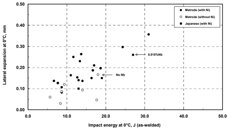
**Figure 5. Relation between as-welded impact energy and lateral expansion at 0°C for T23 SMAW weld metals.**
