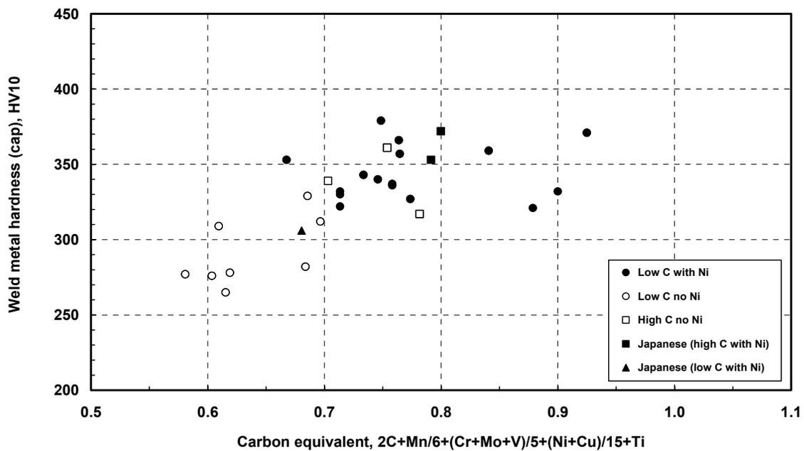
Figure 4. Relation of as-welded T23 SMAW weld cap hardness and carbon equivalent.
