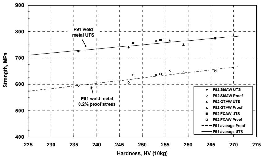
**Figure 1.** Relation between hardness and tensile properties of P92 weld metals, compared with average trends for P91 weld metals.
