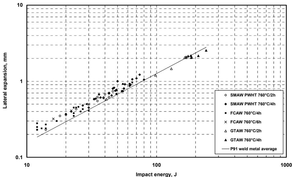
**Figure 3. Relation between Charpy impact energy and lateral expansion of P92 weld metals, compared with average trend of P91 weld metals.**
